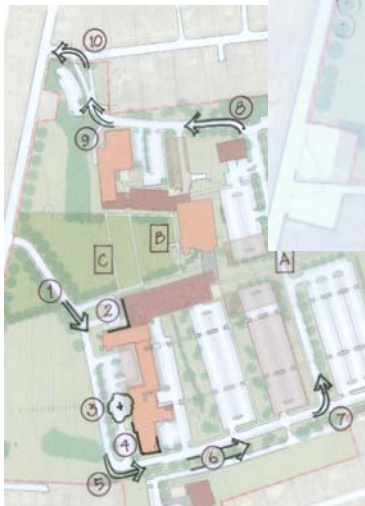
WCA's critique of the bypass concept (left) led to this conceptual layout for an internal loop road (above). With a few minor adjustments, this scheme with its dual drop-offs became the final design for the new campus circulation plan.
